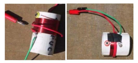
Above right: The 20metre coil: 10 turns of 0.8 mm enamelled wire
