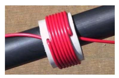
1. Cut the radiating wire to a length of 10.1m. This includes the wire for the coil. 2. Cut a 30 mm length of 42mm diameter PVC pipe for the offcentre\* coil former. - drill two 2mm
