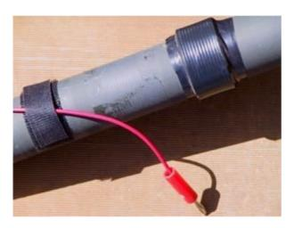
The Velcro patch on the left of the illustration is a simple way of holding the radiating wire captive to stop it unwinding. The top Velcro layer lifts back to release the wire. The black taped over nylon strap on the right of the illustration is a sort of buffer/collar that helps prevent the bottom end of the squid pole from rattling round inside the PVC
