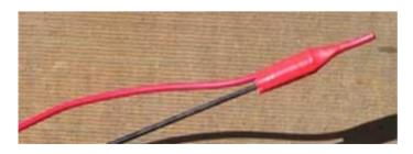
small diameter rawl plug is used to slide firmly over the top of the squid pole after the tiny wire loop at the top of the squid pole is cut off. The radiator wire is taped to the rawl
