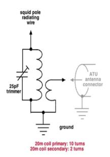
The end-fed half wave squid pole is 'ground independent' with an elevated high current radiation point providing excellent low angle radiation; you'd need a Yagi or a curtain or 4-square array to beat it. The trimmer capacitor is easily adjusted for a flat SWR into a 50 ohm load so it works with no ATU.
